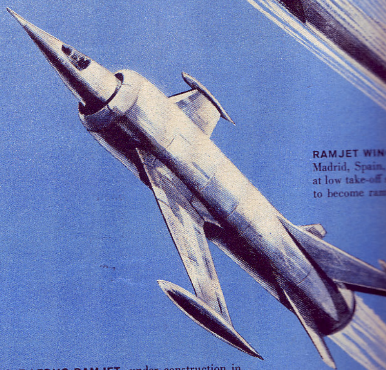
THE LEDUC RAMJET , under construction in France, is a flying tube that serves as the plane's body and becomes a giant ramjet engine at high speeds. It uses jet engines in wings for take-off.
